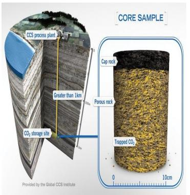
A cutaway of the Earth shows how impermeable rocks cap CO<sub>2</sub> reservoirs. Global CCS Institute
